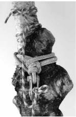
With the tail of the rigging rope defined by a slip knot, attach the rigging rope to the *load.....*
