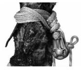
Tuck the tail of the soft eye sling under at least one leg of rope at the back of the tree to keep it away from running ropes and moving *loads*.
