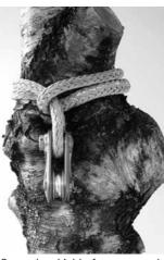
Generate a bight of rope around the standing part by passing the tail back around the tree in the opposite direction.
