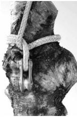
Pass the tail of the soft eye sling around the tree and under the standing part, close to the Impact Block.
