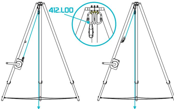
**Fig. 6 –Lifting with the winch (I) –** Using the winch (I), semi-static ropes (EN 1891) with a diameter between 10 and 12 mm can be manoeuvred to lift a maximum load of 1.5 kN for the entire length of rope.
